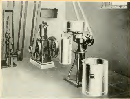
Up-to-date Dairy with Oil Engine and Cream Separator
