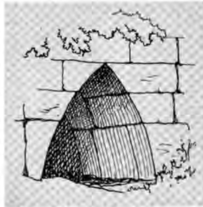
PREHISTORIC GRECIAN POINTED ARCH Not constructed on the true principle.
